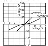
9. Off state leakage current
