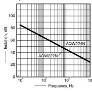
14. Insertion loss characteristics (50  $\Omega$  impedance)
